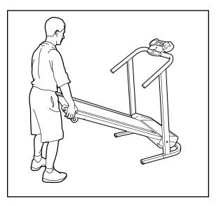
2. Move your right hand to the position shown and hold the treadmill firmly. Raise the treadmill until the latch pin is aligned with the hole in the left upright. Slide the latch pin into the hole. Make sure that the latch pin is inserted as far as possible into the hole. Lock the pin by pressing the end of the pin into the slot in the storage latch as shown in the inset drawing.
